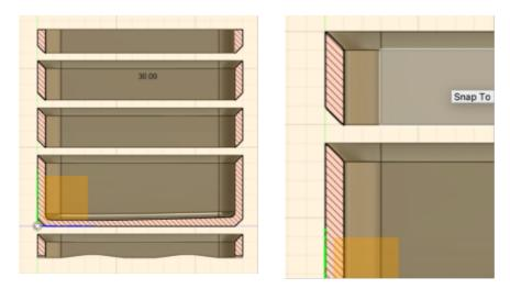
Between these layers, a rubber layer would be placed to maximize the watertightness between the layers. To make the attachment between the layers more sturdy, and the watertightness maximal, clips are attached on the sides of all layers, connecting the layers and increasing the force applied between the layers. We considered many kinds of latches and clips to connect the layers. After some deliberation we found that the ideal material for these clips would be stainless steel.
