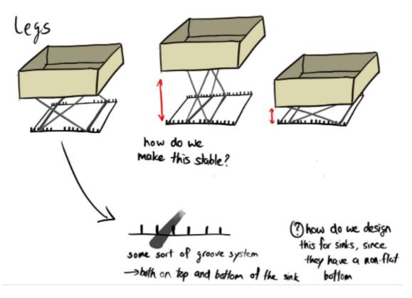
These x-shaped legs were, however, instable and too complicated and breakable. In the next iteration, the product consists of multiple layers, one of which has a bottom with a drain. This layer can be moved to different heights by rearranging the layers. There would also be a layer that remained on top which was fitted with flaps to prevent dishes from falling between our product and the sink.
